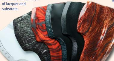
Films decorated with Norilux® FastCure 1 can be 3D formed after the drying process by high pressure forming or thermoforming.
