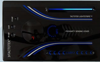
Tactotek injection molded structural electronics panel (IMSE)
