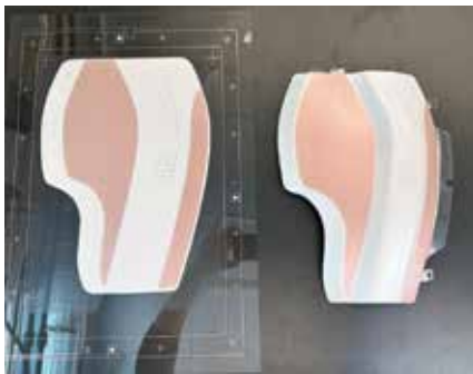
Screen printed PC film (left), high pressure formed film (right)
