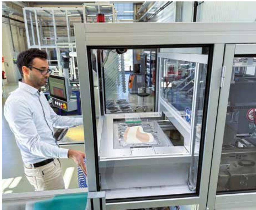
Proell Center – Niebling high pressure forming of screen-printed films
