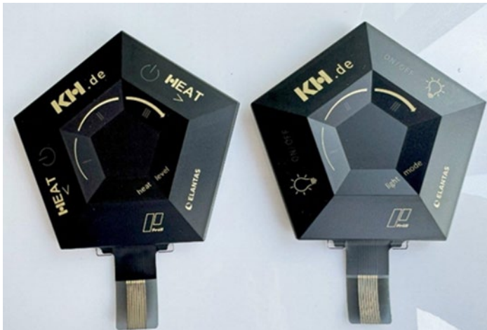
Picture 2: Functional IMD/FIM demo part from KH-Helmbrechts. Non-conductive IMD/FIM ink systems are used for pre and back printing of the printed conductive silver pastes.
