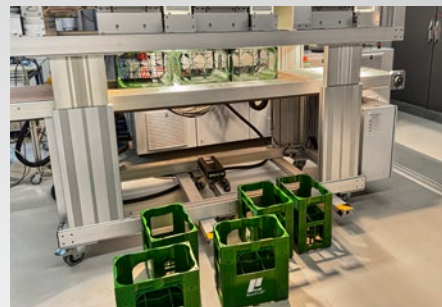
Drying with a "Multiple-IR-Curing" NIR module.
