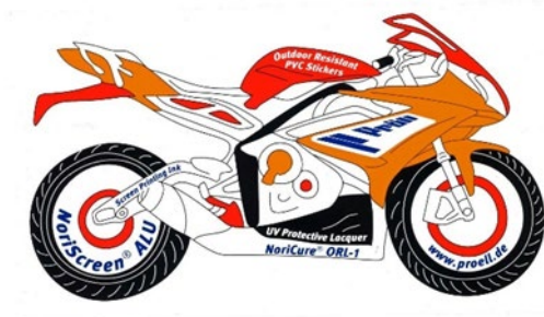
Picture 6: Outdoor-resistant PVC sticker printed with NoriScreen® ALU screen printing inks and protected with NoriCure® ORL-1/001.
