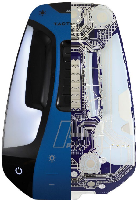
Picture 2: Picture collage - functional IMD/FIM demo part from TactoTek. Non-conductive IMD/FIM ink systems can be used for back printing of the printed conductive pastes.
